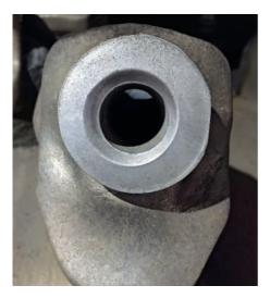
HT22 quick-change toolholder system after a service period of at least 50 operating hours with a W6/20A pick.
