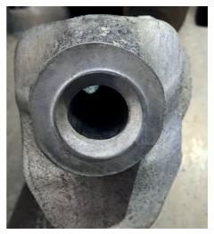
HT22 quick-change toolholder system after a service period of at least 50 operating hours with a W6/20A<sup>2</sup> pick.
